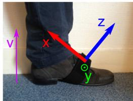
(a) Definition of the axis for the XSens<sup>TM</sup> sensor located at the left foot
