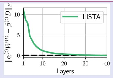
40-layers LISTA network trained on a 10  $\times$  20 problem with  $\lambda = 0.1$ The weights  $W^{(t)}$  align with D and  $\alpha, \beta$  get coupled. Restricted parametrization : Only learn a step-size  $\alpha^{(t)}$
